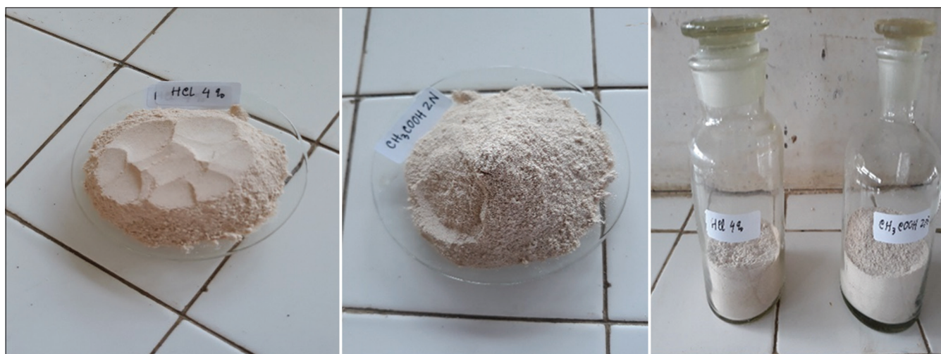
Figure 1: Extract of chicken eggshell from maceration of 4% HCl and CH 3 COOH) 2 N
